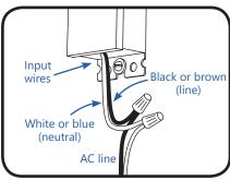
Connect the AC line to the black or brown (line) and white or blue (neutral) input wires of the power supply using suitable wire connectors.
