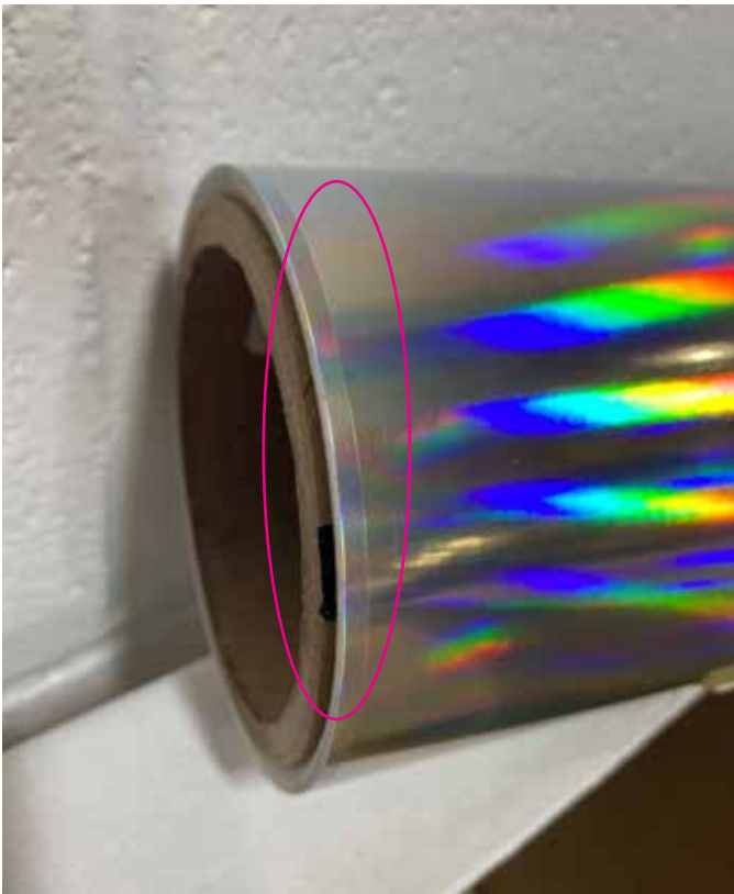
Example of shim line located at the edge of a 30" roll:
