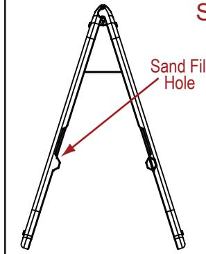
Each sign frame has two fill holes, one on each side of the frame.
