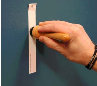
FIGURE 3 Adhering Film Strips
