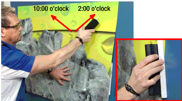
FIGURE 18 Squeegee with the 10:00 and 2:00 O'Clock Position; End Stroke Past Film Edge
