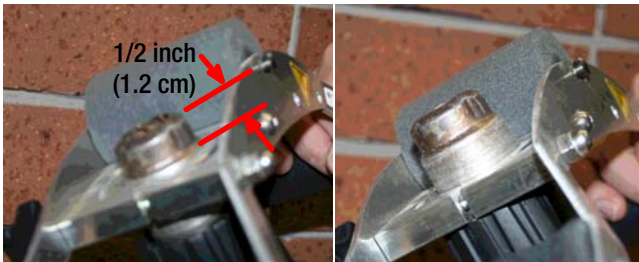
FIGURE 23 Positioning Heat Gun Nozzle in Heat Gun Holder
