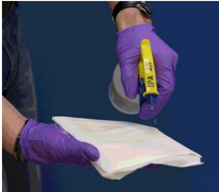
FIGURE 6 Soaking a Lint-free Cloth
