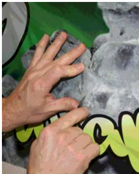
FIGURE 36 Cut Away Film a Little at a Time
